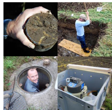
Soil sample, soil profile of the test field, sampler for flow proportional sampling, drainage manhole.
