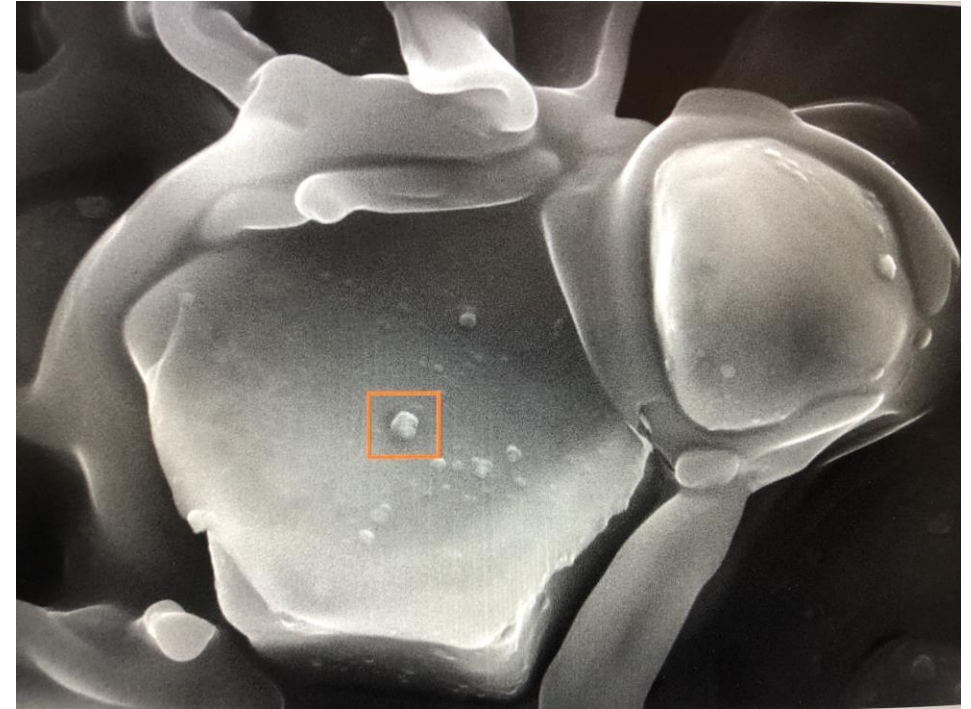
Scanning electron micrograph (SEM) showing a particle of \text{TiO}_2 in yellow box on a particle of food.
